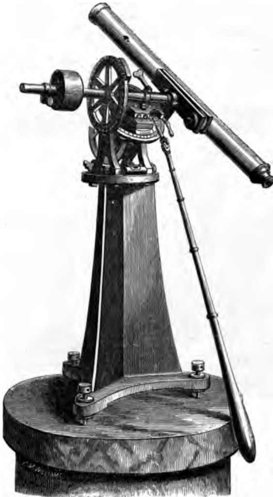
GERMAN EQUATORIAL. ( By Horne and Thornthwaite. )
